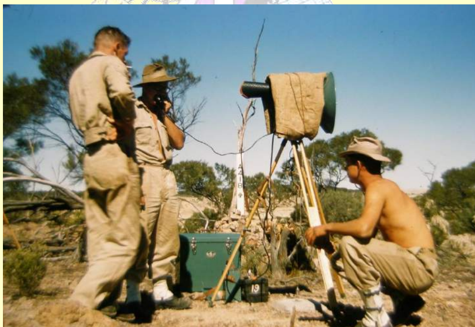
At station A 418 - the tellurometer MRA1
