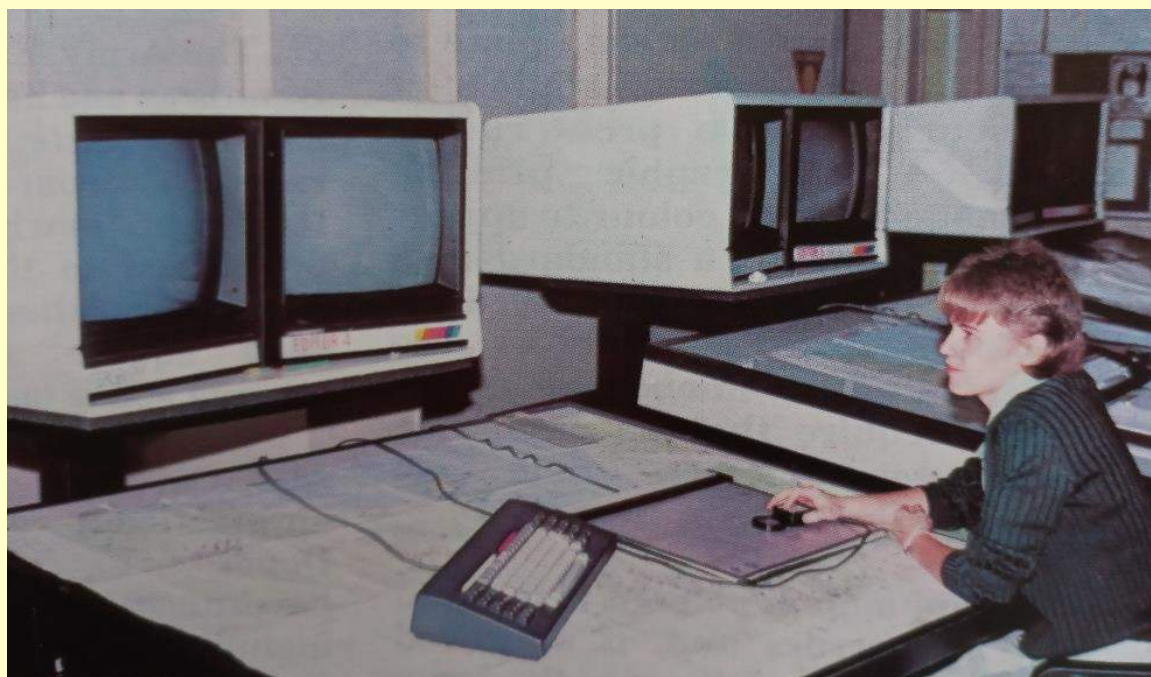
Army Survey Regiment, Bendigo VIC - 1991 Technician Cartographic Sapper Jodi Bowman (from NSW) editing digital topographic data as part of cartographic completion on a graphic edit workstation - part of Automap 2 computer assisted mapping system
