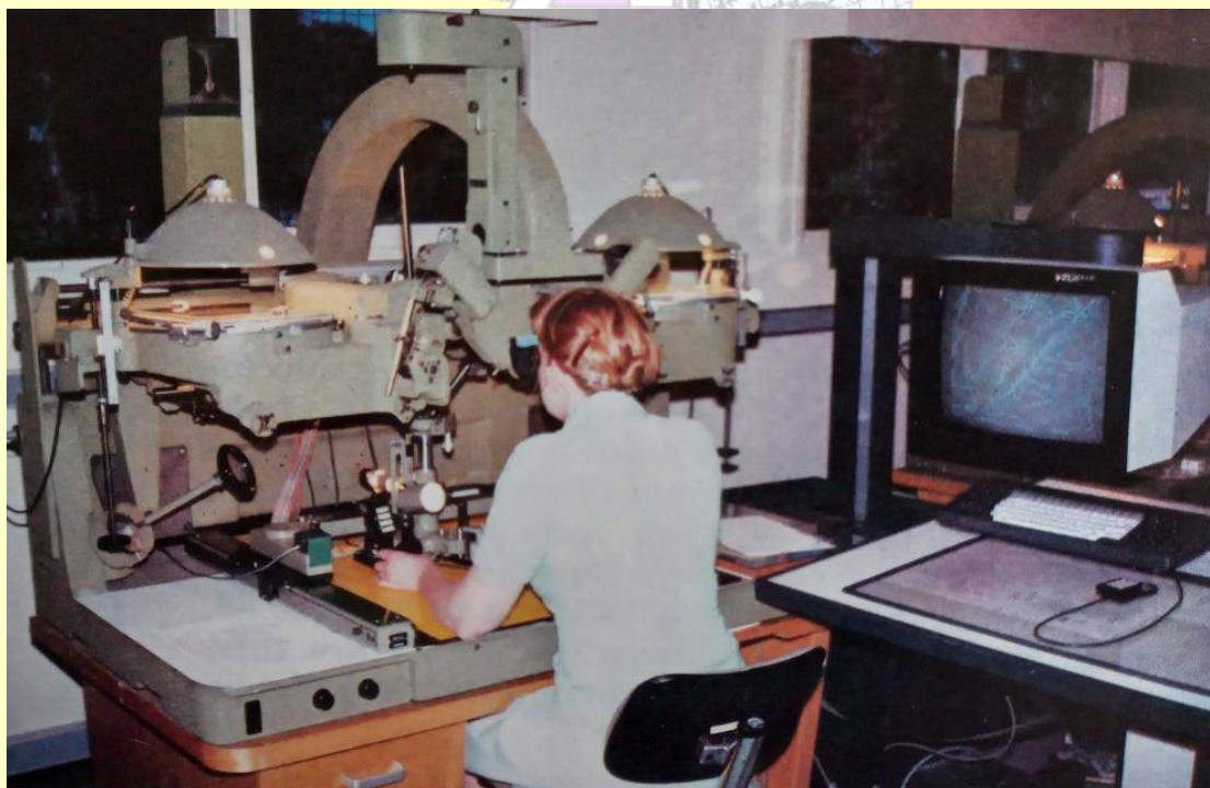
Army Survey Regiment, Bendigo VIC - 1991 Technician Cartographic Sapper Jeanette Lane (from NSW) plotting three-dimensional digital topographic data from aerial photographs using a computer assisted stereographic photogrammetric plotter - WILD B8 part of Automap 2 computer assisted mapping system
